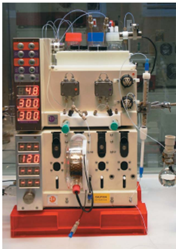
Fig. 1 VapourTec R2 + and R4 combination flow reactor.
